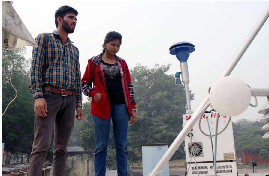
▲ CEEW's L.S. KURINJI at the Ambient Air Quality Monitoring Station, Aurobindo Marg, New Delhi, to ground-truth satellite readings on pollution activity with on ground readings. 2019.
