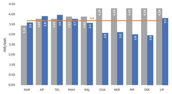
**The higher capacity in medium-low WPD sites will result in a higher LCOE and lower energy production.** Figure 7 shows the state-wise average LCOE for wind power plants and the average cost of non-RE power.
