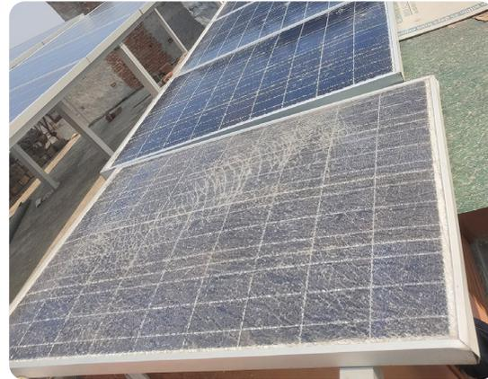
If a **shattered module** is still attached to system, it causes low power production and is a high safety concern
