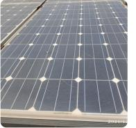
**Deposition of dust** layer due to improper cleaning or poor water quality resulting in low performance Possible causes poor water quality, improper cleaning
