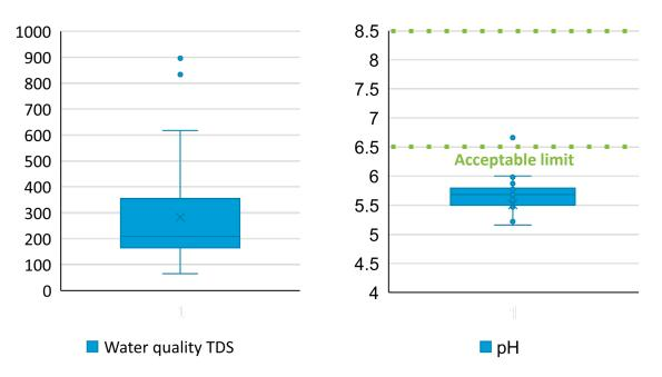
The issue of scaling / cementation on PV modules may be due to poor quality of water and improper cleaning of modules
