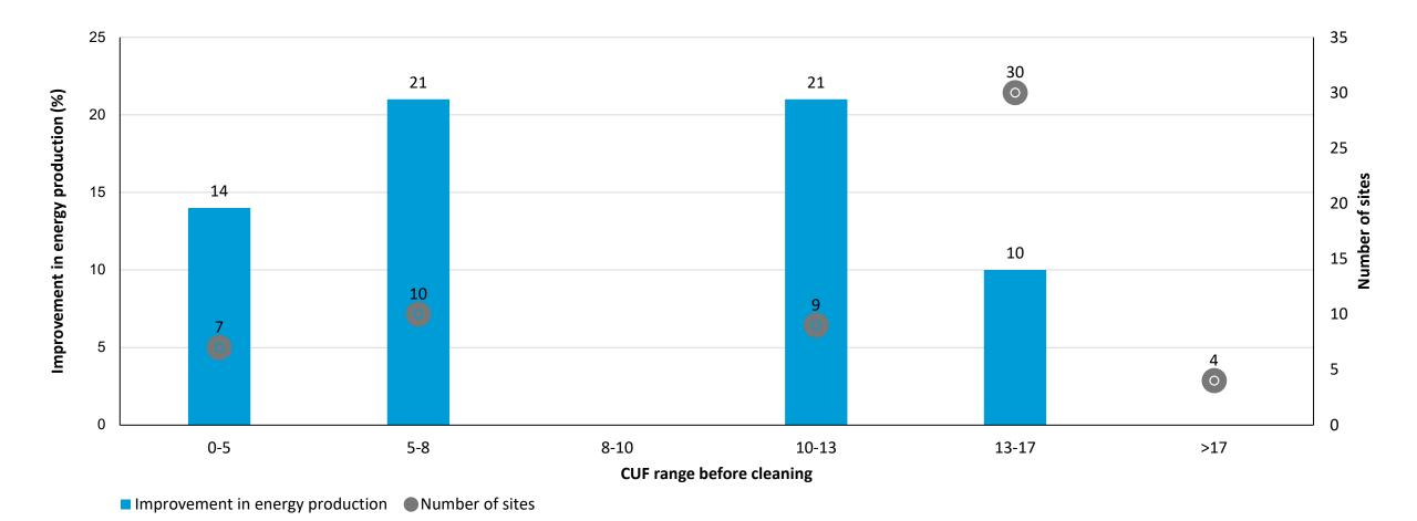
System performance improves by more than 10% with onsite cleaning. Due to poor air quality, modules have to be cleaned periodically. There is a further scope for improvement in performance, if a proper O&M system is in place.
