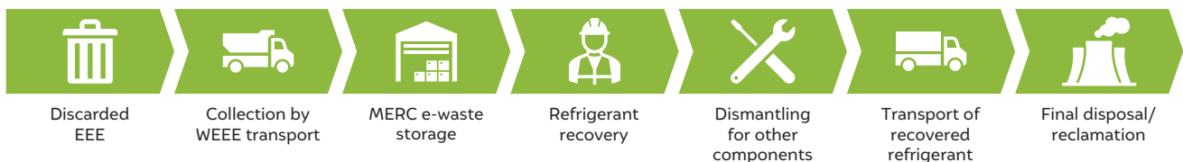
Figure 5 Mechanism followed in South Korea for collecting refrigerants at the EOL of a cooling appliance
