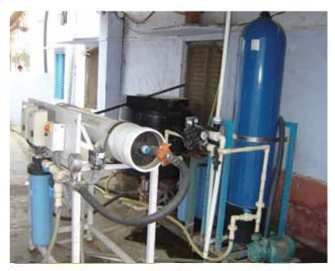
Figure 4: Barefoot College's solar RO desalination unit,Kotri, Rajasthan<sup>26</sup>Source: (Barefoot College)<sup>27</sup>
