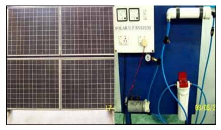
Figure 9: BARC solar powered water purifier based on ultrafiltration Source: (BARC)<sup>48</sup>
