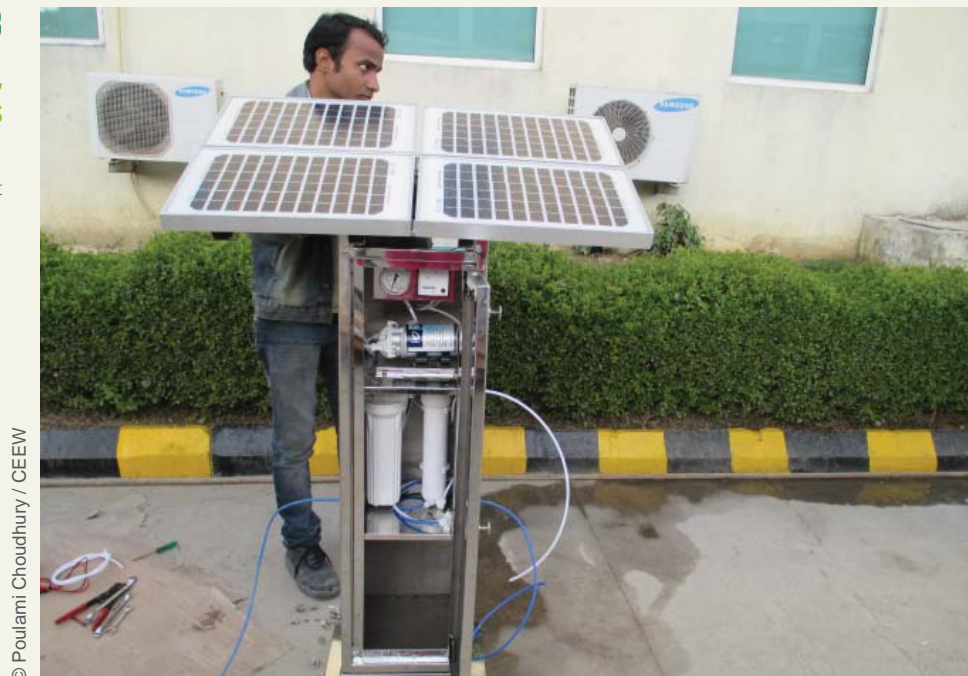
FIGURE 3.3 Solar PV-RO Purifier (10 L/h), Jakson Solar Solutions
