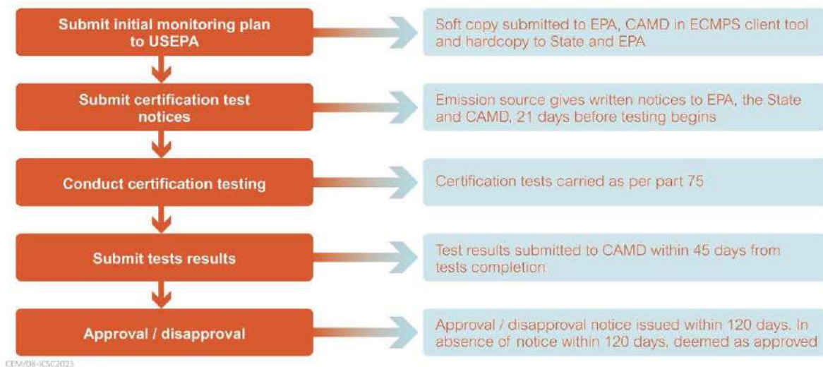
Figure 8 Process flow of CEMS testing and approval as per USEPA in the USA (USEPA, 2009)
