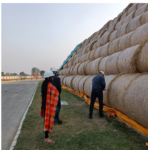
CEEW's Kurinji Kemanth in discussion with Verbio team on the importance of raised platform (left); waterlogging was seen affecting base layer of stack (right).
