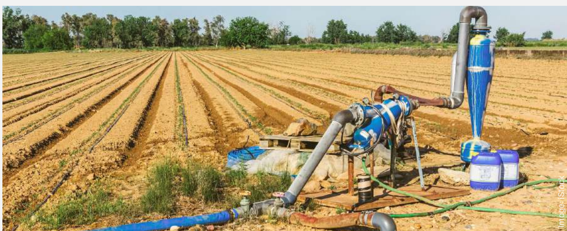
Pump for supporting drip irrigation on farm.
