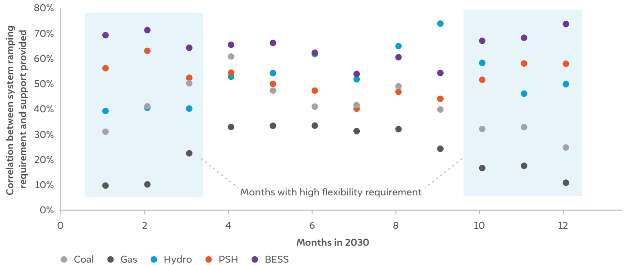
Figure 11 BESS supports high system ramping requirements
