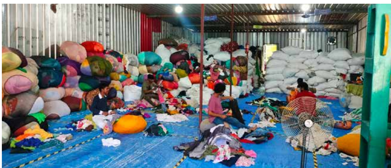
Manual sorting of textile waste by colour and pattern at a textile recovery facility (TRF) in Maharashtra.
