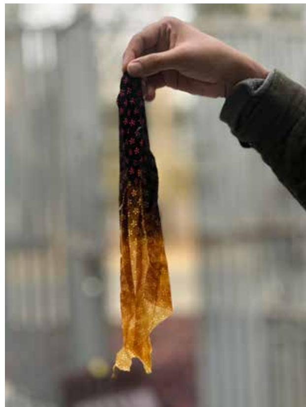
Sample of bleached, colour-sorted pre-consumer textile waste prepared for recycling into fibres, observed during a field visit in Haryana
