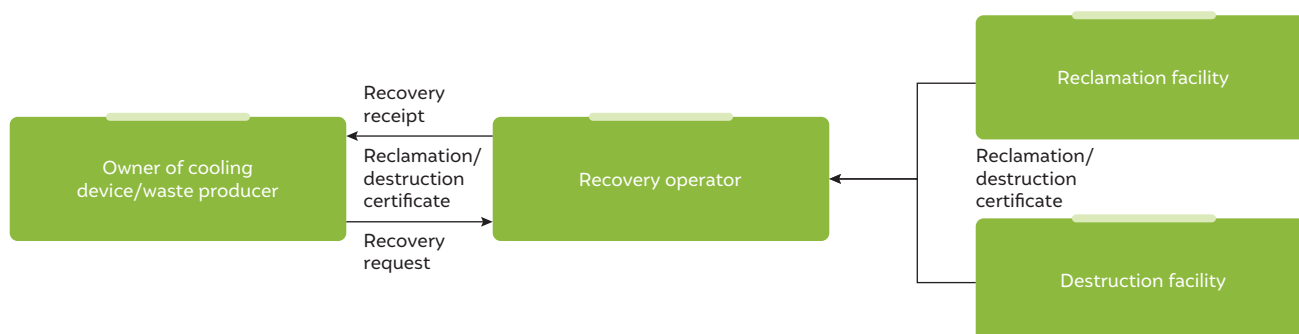
Figure 4 Refrigerant recovery, reclamation and destruction certificate flow in Japan
