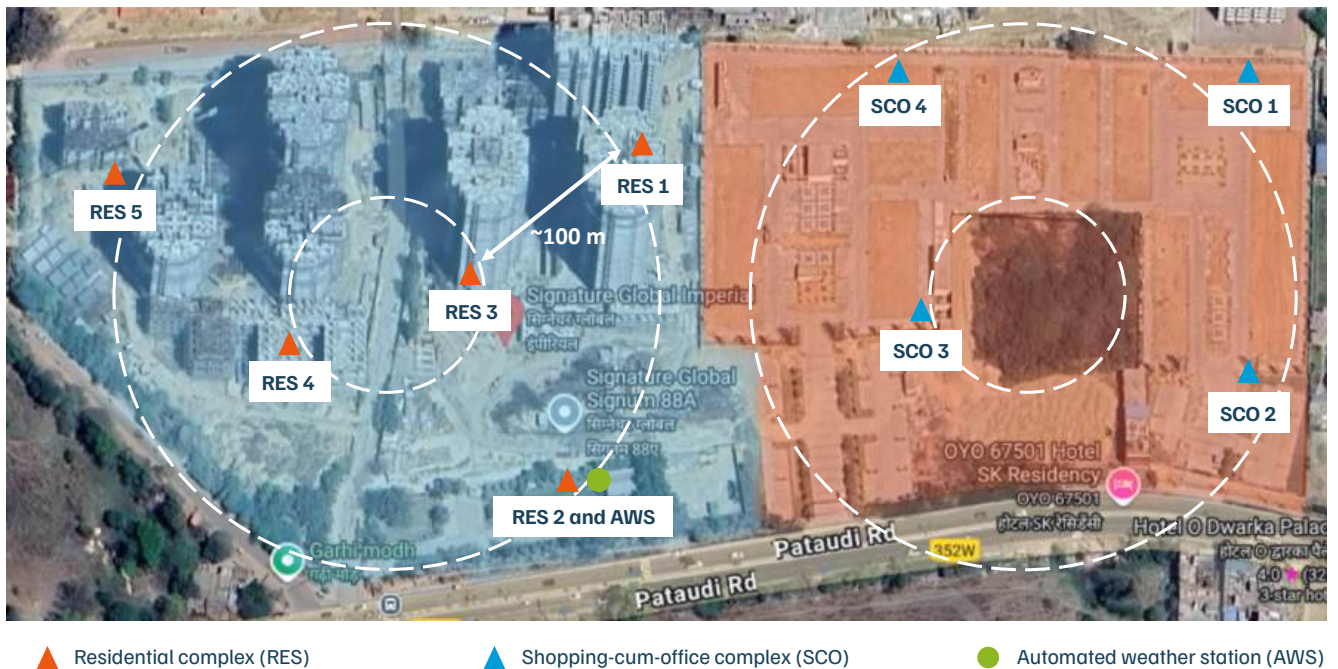
Figure 2. A representative visual of the monitoring network showing the placement of the nine low-cost sensors and the automated weather station arranged in a concentric circle pattern
