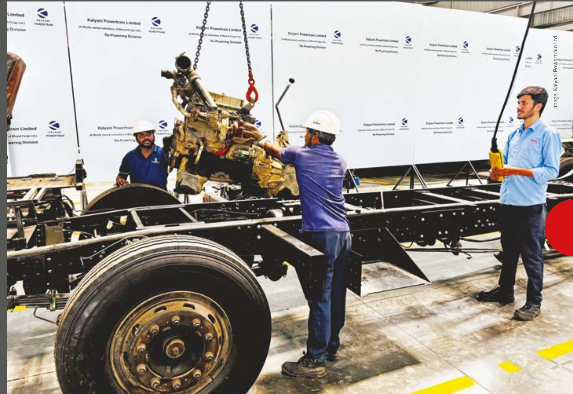
▲ A team of technicians carefully removes ICE components from the bus, modifies the chassis, and installs the EV kits, to effectively convert the bus into an extended-life electric bus.
