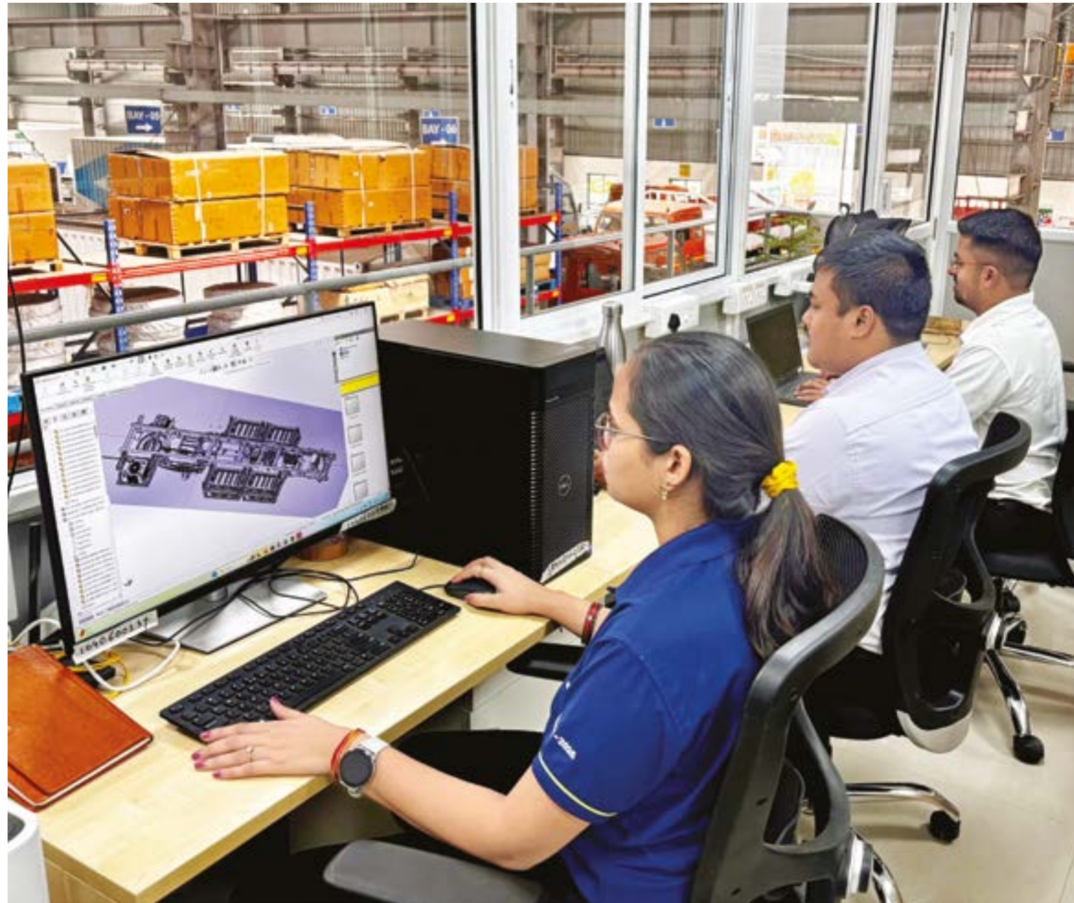
▲ Team of retrofiters developing 3D models of ICE vehicles to design parts for its retrofitment.
