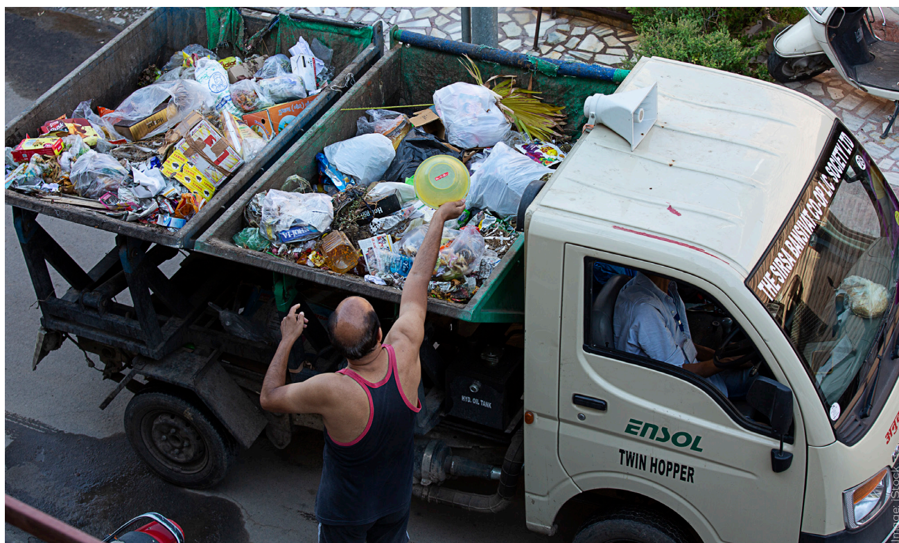
Indian cities typically deploy ICE-based light commercial vehicles with a payload capacity of 300–1000 kg for door-to-door waste collection.
