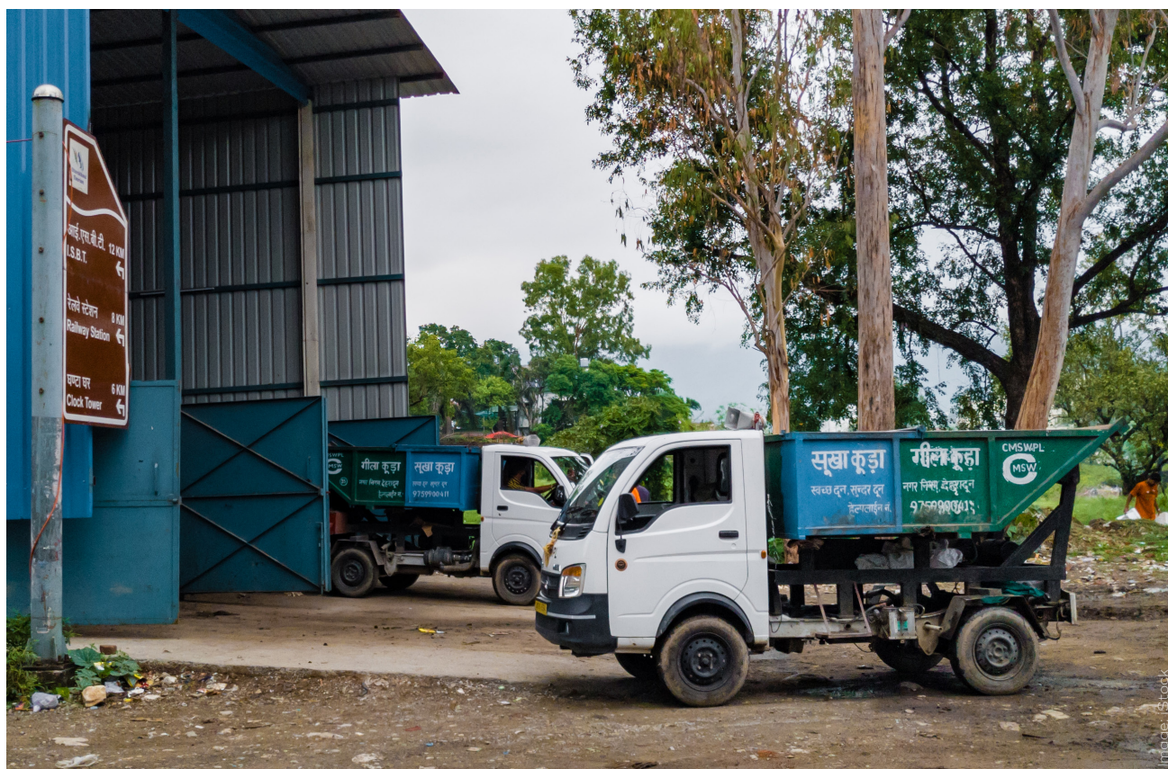
Door-to-door waste collection vehicles must have robust hydraulic tippers to empty waste at transfer stations or landfills.
