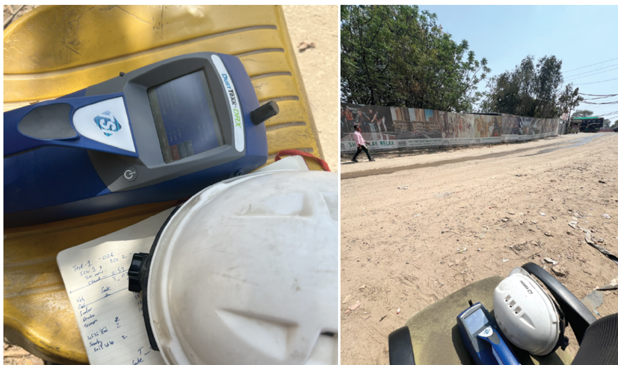
Monitoring particulate matter (PM) concentrations along a ~100 m approach road using a TSI DustTrak DRX.
