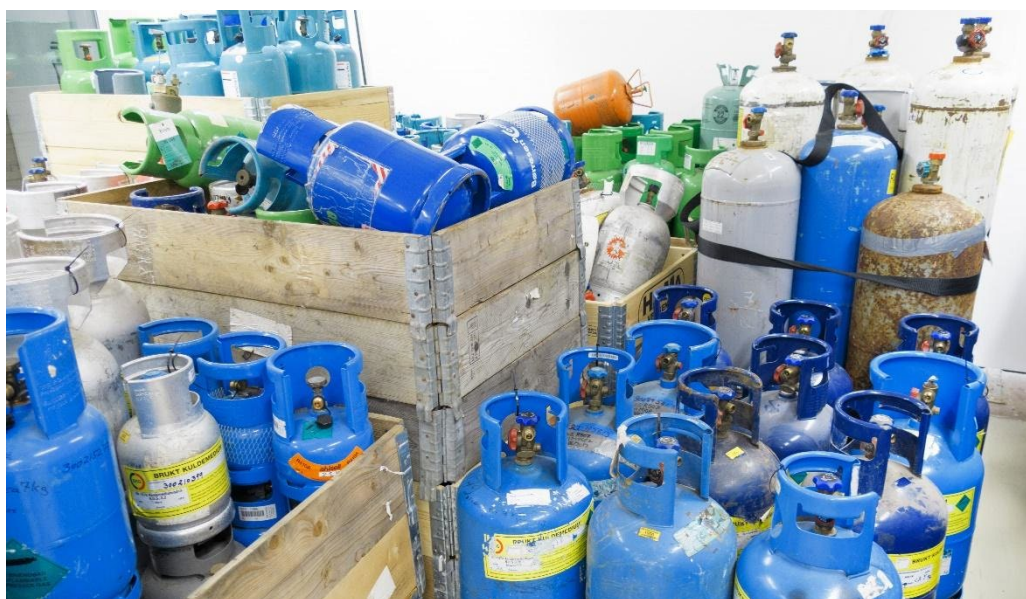
Figure 25: Cylinders of collected waste refrigerants ready for analysis and further treatment.
