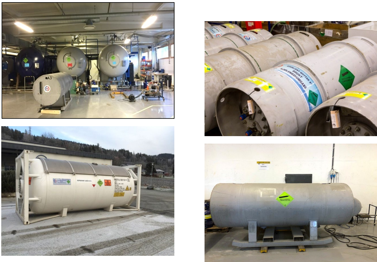
Figure 28: Tanks for transportation of recovered refrigerants
