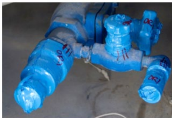
Figure 14: Sealed valves on tank before transport and weighing of tank containing recovered refrigerants
