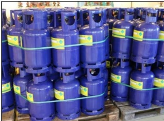
Figure 29: 27,2 L refillable cylinders for non-flammable refrigerants. IBC container.
