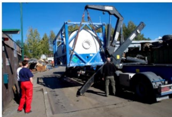
Figure 14: Sealed valves on tank before transport and weighing of tank containing recovered refrigerants
