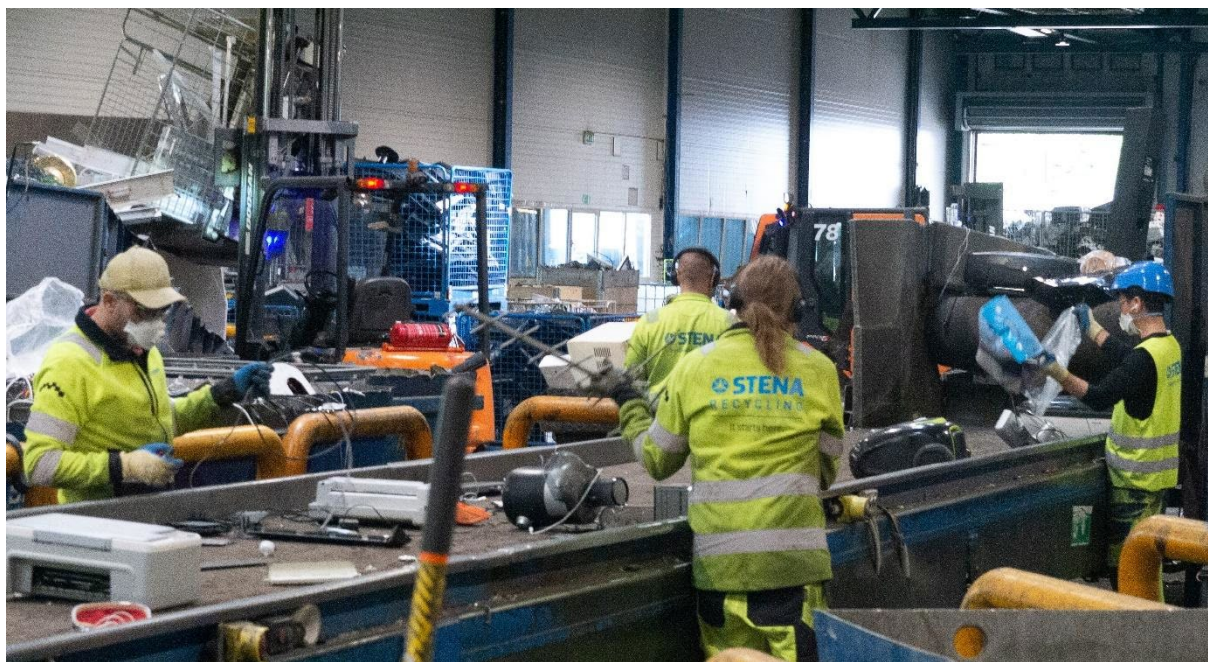
Figure 20: Sorting and treatment of waste from electrical and electronic equipment (WEEE) at Stena Recycling.
