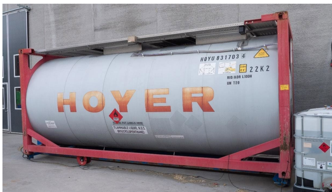
Figure 22: Tank at Revac containing a mixture of CFCs and hydrocarbons. The gases are collected from insulation foam in old household fridges and the tank has been readied for transport.
