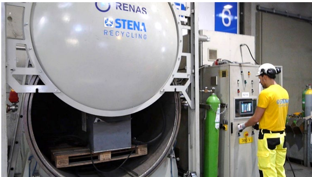
Figure 32: 100% recovery of SF 6 in GIS by use of a vacuum chamber.
