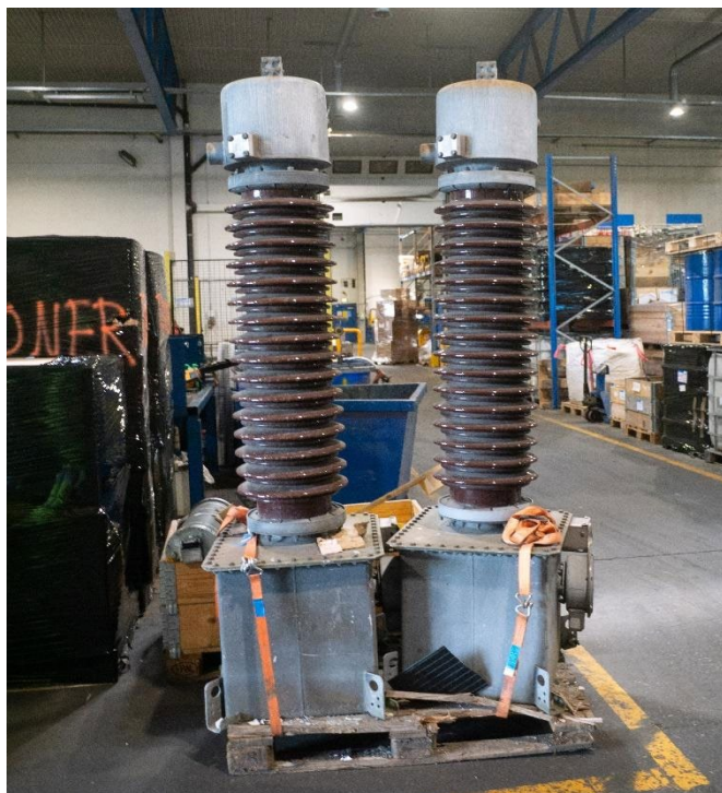
Figure 18: Equipment from power supply awaiting recovery of SF 6 .
