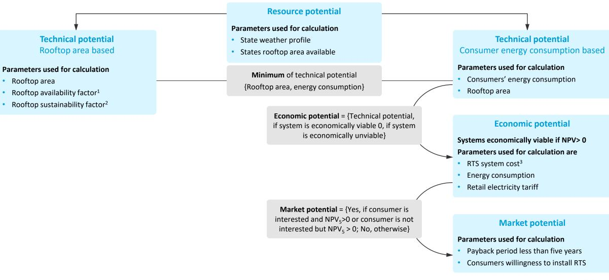
Notes: 1. Rooftop availability factor determines the availability of roof space for installation after accounting for shading, obstructions, and other constraints.
