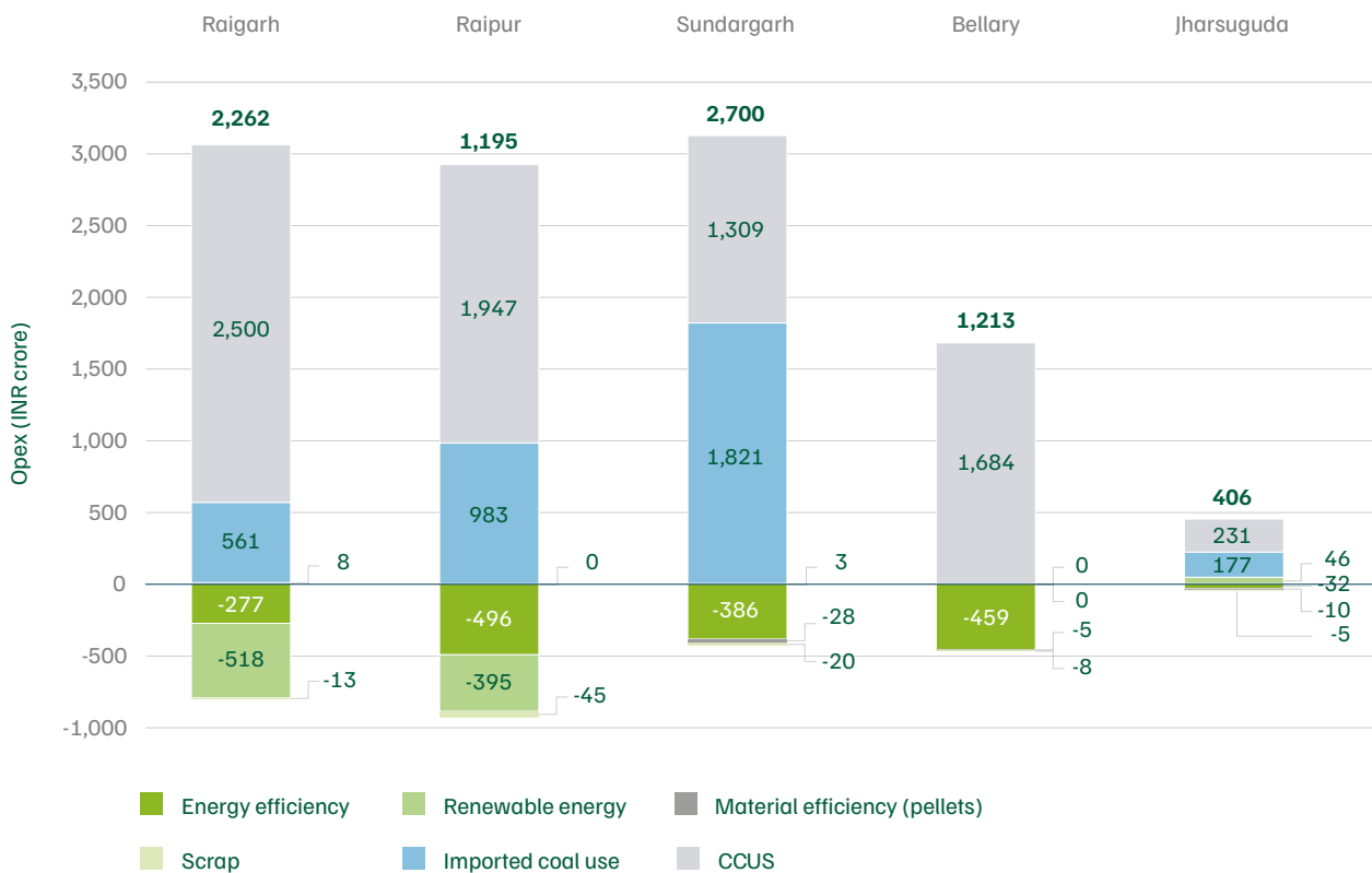
Figure 23. CCUS and adopting imported coal use have the highest operating expenses amongst measures
