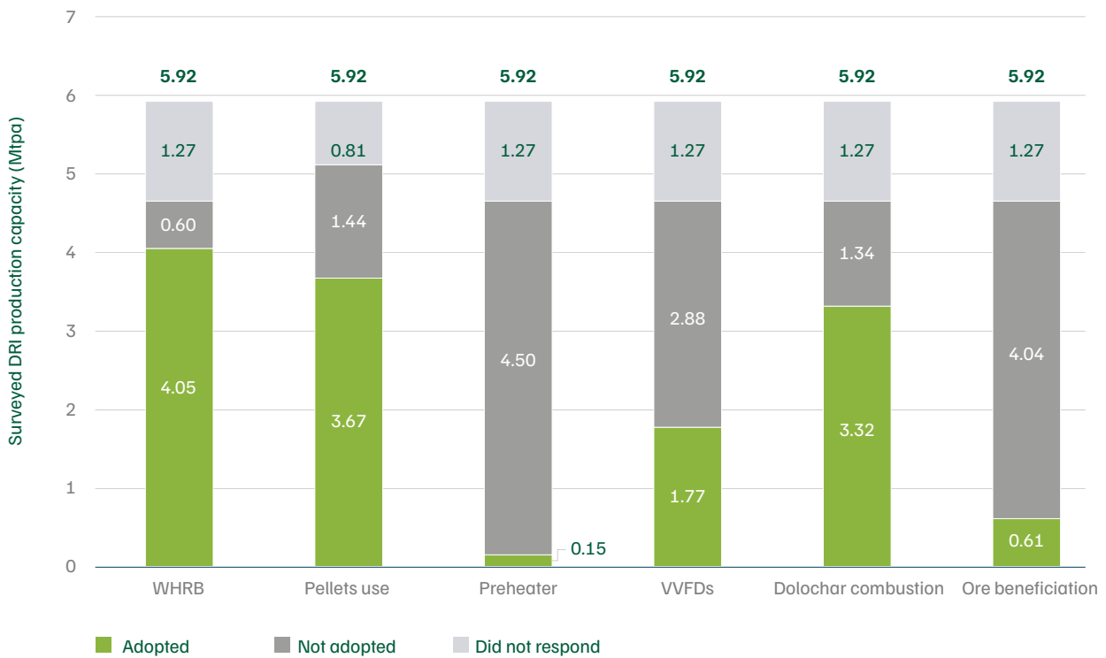
Figure 14. Pellet use, waste heat recovery boiler (WHRB), and dolochar combustion are the most adopted energy efficiency (EE) measures in the five clusters
