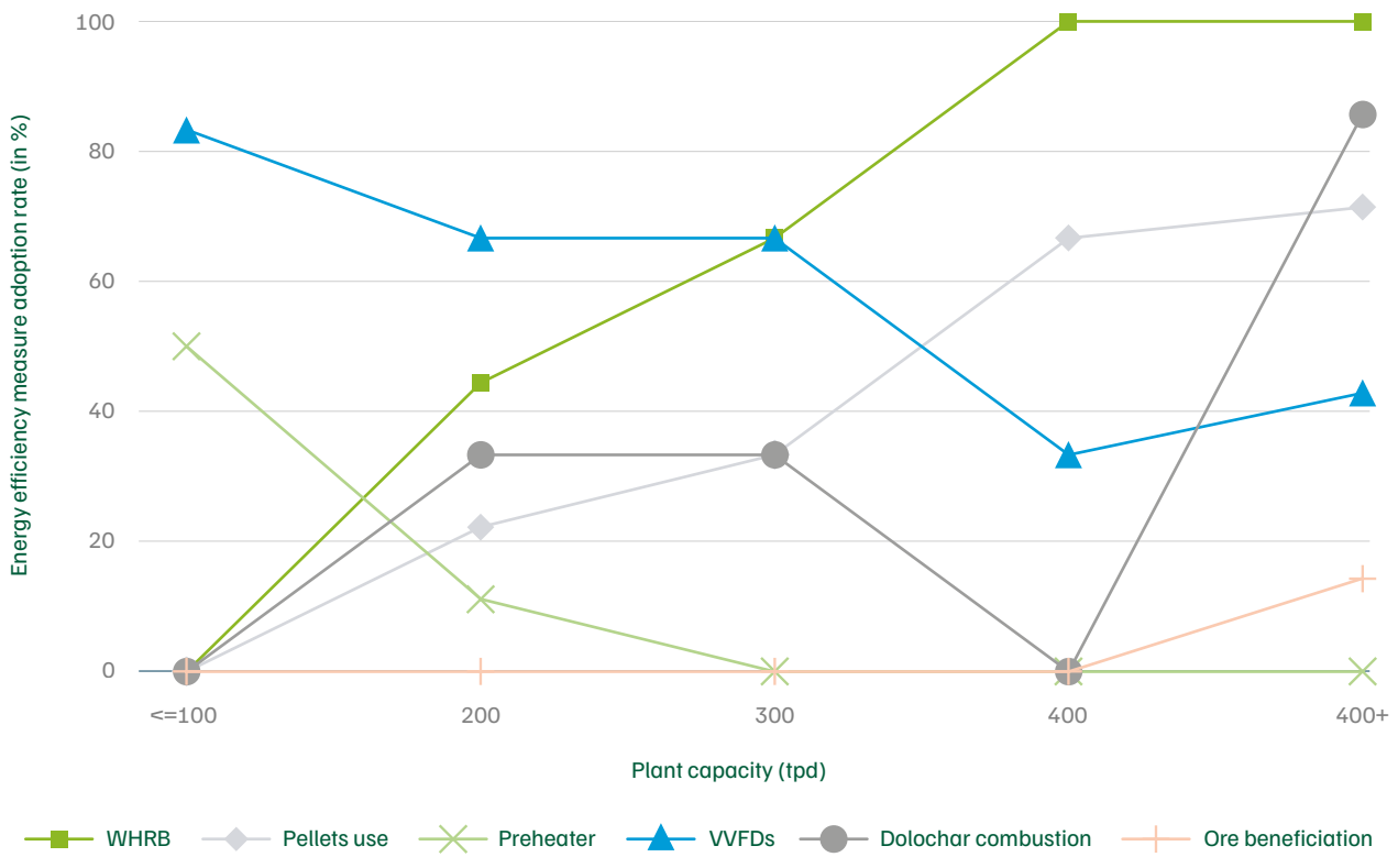
Figure 15. Adoption of EE measures usually increases with the plant capacities of the units surveyed, except for ore preheating and variable voltage frequency drives (VVFD)
