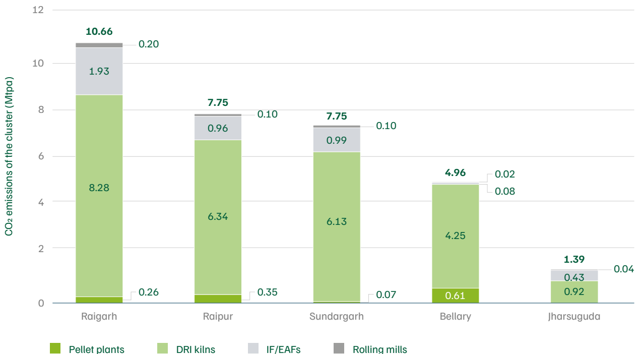
Figure 19. DRI process accounts for the highest share of total emissions from a steel cluster
